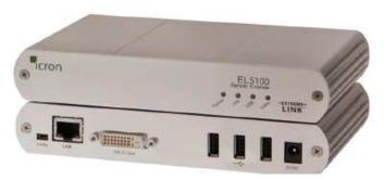
The EL5100 KVM Extender, powered by ExtremeLink™ technology, lets you place a computer up to 330 ft (100 m) away from the workstation area, connected with a single inexpensive Cat 5 (or better) cable. The system supports full HD video and USB 2.0, including control of the keyboard, mouse, webcam, flash drive, speakers, microphone and other USB 1.1 and USB 2.0 devices.
